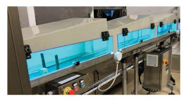
The specific design is flexible enabling it to adapt to any type of roller conveyor belt. Depending on the conveyor belt specification, the system design allows it to work with 1-8 lamps as required. The larger the surface or the faster the conveyor belt the more lamps will be required.
